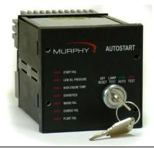
A proven industry standard, the Autostart 700 control module provides fully automatic start up, load transfer, fault monitoring and shutdown of a stand-by diesel generator, pump or stationary engine.
